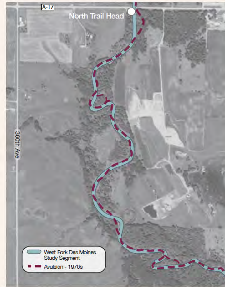
Figure 9 The current aerial photograph of the North Trailhead Access are shown here along with the mid-1970’s channel centerline (shown in pink). Few changes in channel location occurred during this fifty year period. However the channel is creating two avulsions. These cut-off sections are shown with a dashed line. The main flow of the channel will eventually occupy these new channel areas.
