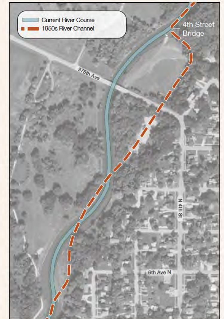
Figure 3 By the mid-1970's the West Fork Des Moines River channel and the 4th Street Bridge had been relocated. One section of the former channel (circled) still retains groundwater.
